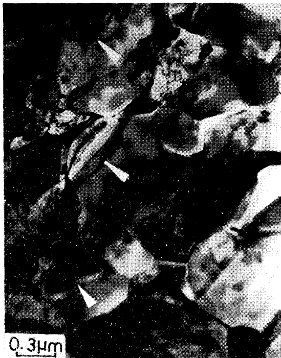
Photo. 8. TEM taken from the specimen annealed at 650°C for 10 min after 95% deformation. Arrows show \beta' -Cu 3 Ti particles.
