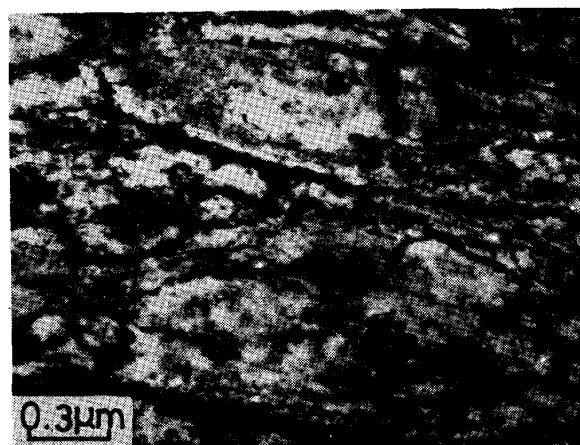
Photo. 2. Cell structure in the 95% deformed specimen, TEM.
