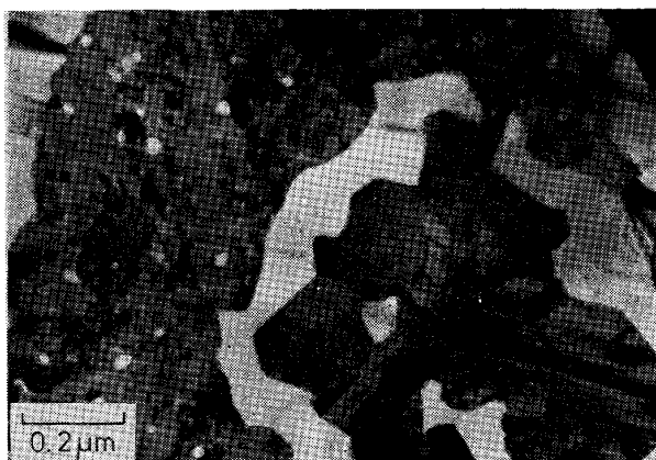
Photo. 5. Phase transformation of metastable phase into stable Al and Ge crystals in Al_{50}Ge_{50} alloy.
