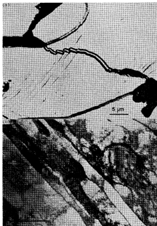
RD-ND section, (a) 10% rolled, (b) 40% rolled. Photo. 5. Optical micrograph (a) and electron micrograph (b) of microbands in rolled steel 23) .
