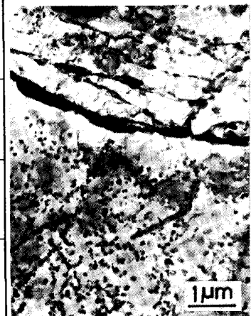
Photo.1 Electron micrograph of 11%Cr specimen ruptured at 550°C and 25kgf/mm 2 for 420h
