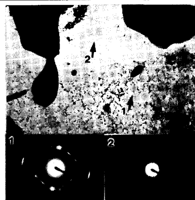
Photo.1 TEM observation and diffraction pattern of precipitates (AlN) and amorphous in N-added capped steel (380°C×15hr)
