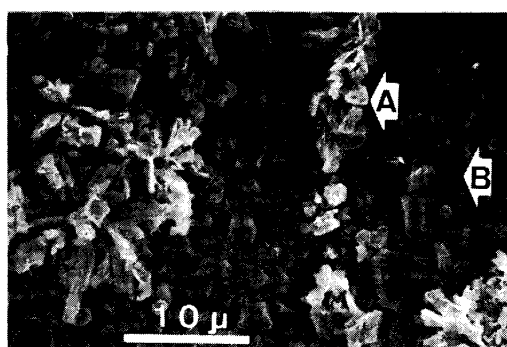
Photo.1 Two types of Fe-Zn alloy phase observed in Steel A.
