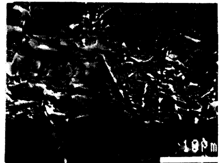
Photo.1 SEM Image of phosphate coatings on Low-Pb galvanized steel after 2T bend test
