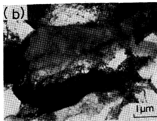
a) optical micrograph b) transmission electron micrograph Photo. 2. Microstructures of an OLAC plate. (0.07C-1.59Mn-0.03Nb-0.07V, 15 mm)
