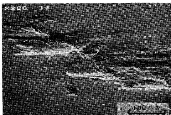
Photo. 9. Photograph of the surface of grain roll of F5 stand in a production mill.
