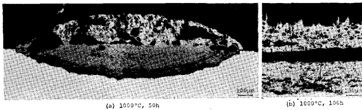
Photo. 3 Cross sections of oxide scales formed on SUS 430 steel heated at 1000°C for 50 and 100 h, respectively in air.
