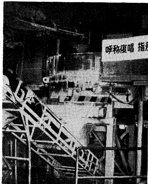
Photo. 5. Mixer and charging and discharging conveyor for casting materials.
