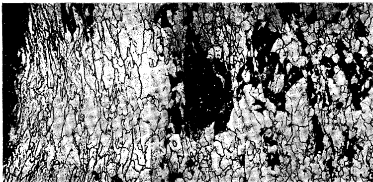
Photo. 1 Crack formation within pearlite particle
