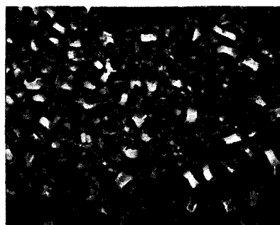
Photo. 2 SEM micrograph of phosphate crystal on Fe-Zn-Sn(0.23%) alloy as outer layer
