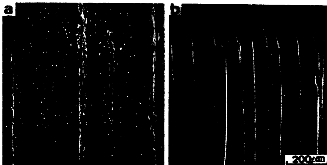
a: Borided die, b: Unborided die, Number of drawn wire with same die: 60 pieces, d : 4.990 mm, l : 112 \pm 0.3 cm, v : 5.14 m/min, r : 3.4%, L : Machine oil.
