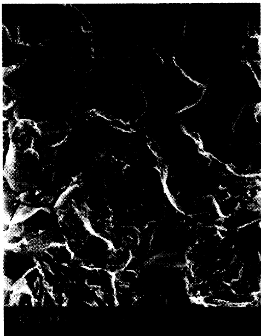
Photo. 4. Fractograph of 123 steel. \Delta K=108\text{kgf/mm}^{3/2} , in pure water bubbling \text{N}_2 gas, 0.167 Hz.
