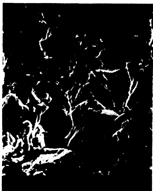
Photo. 3. Fractograph of 104 steel. \Delta K=56 \text{ kgf/mm}^{3/2} , in 3% NaCl solution bubbling air with zinc sacrificial anode, 0.167 Hz.
