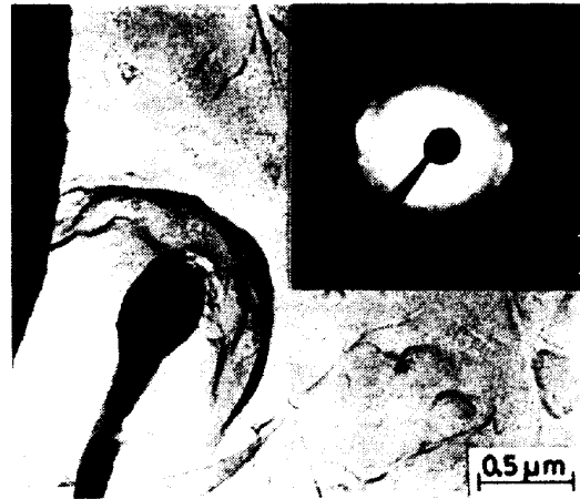
Photo. 2. Electron micrograph of BN extracted from fracture surface of bend specimen of 20B steel.
