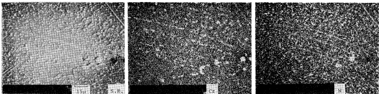
Photo. 4. Characteristic X-ray images of carburized layer in KSN ruptured at 900°C after 1360h in Reducing Gas (R.G.).
