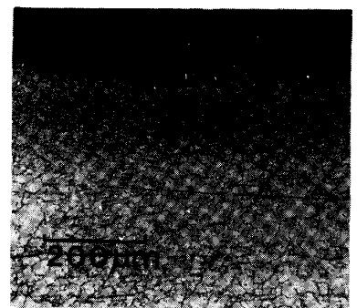
Photo 1. Microstructure beneath the surface of quenched strip (1100°C 40%)
