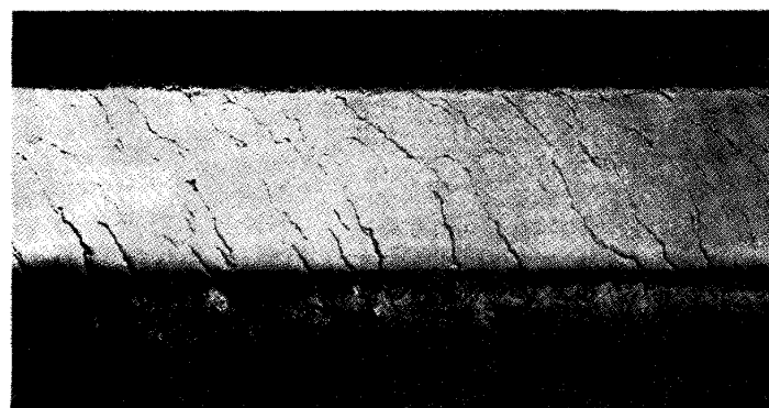
Photo. 3 Head checks at the gage corner
