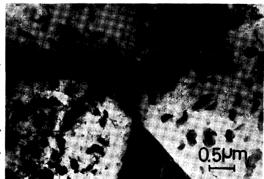
Photo.1 Electron micrograph of G1-steel reheated at 550°C for 10 4 hrs after tempered at 700°C.
