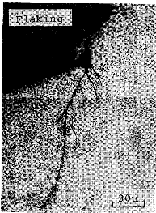
Photo. 3. Platelike carbides developed in thrust specimen tested at 120°C.
