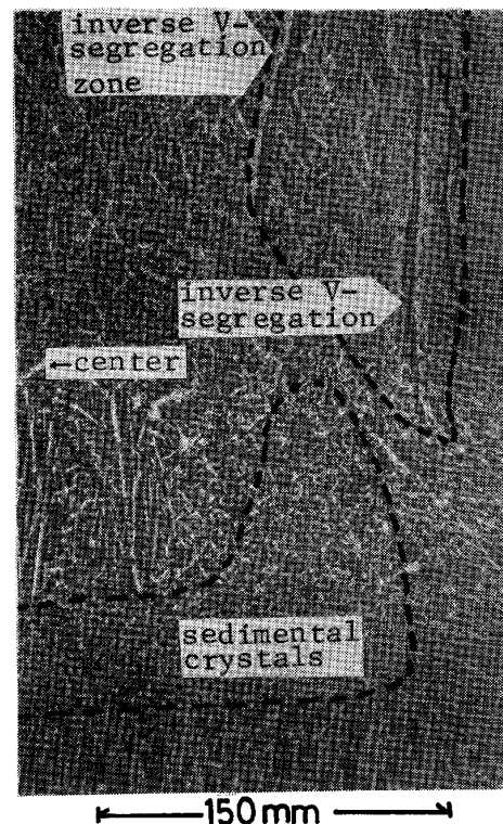
Experimental series : (1) Size of ingot : 720mm×2300mm×700mm H (10 t) Heat insulation type : II
