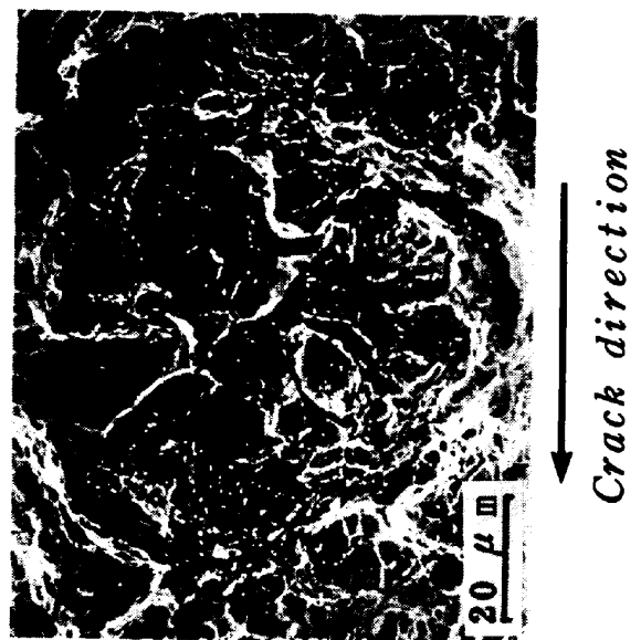
Photo. 6. Intergranular crack origin and crack growth by microvoid coalescence mode for specimen LRS tempered at 530°C.
