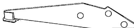
Fig. 8. (Engine support) : Service inflection stress has not allowed to use high strength steel reduced thickness.
