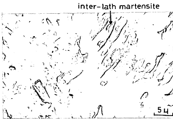
Photo. 2. Plastic-carbon 2 stage replica image of 0.07%C-0.5%Si-2.0%Mn-0.3%Cr-0.10%Ti steel coiled at 550°C.
