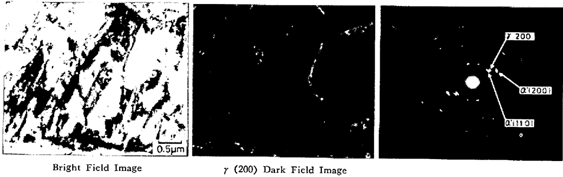
Photo. 5. Transmission electron micrographs showing the presence of retained austenite films between the martensite laths (0.06%C-0.7%Si-1.4%Mn, FT 820°C).
