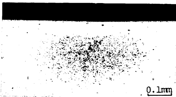
Photo. 1. Dark etching constituent developed in SNCM 420 carburized steel. P_{max} = 540 kgf/mm 2 , Stress cycles: 6.98 \times 10^6 .
