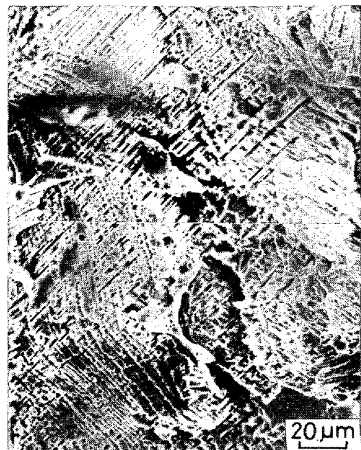
Photo. 4. Preferential attack along slip lines on the fractured surface of the specimen water-quenched, followed by sensitization at 823 K for 7.2 ks after strained to 3.0%.
