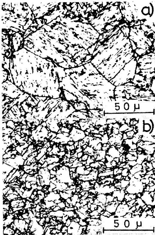
Photo. 1. Optical micrographs of specimens : a) quenched from 900°C(1h) and b) double-quenched from 900°C(1h) and 780°C(1h).
