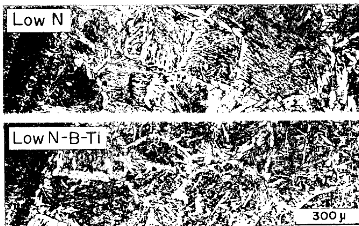
Photo. 1. Microstructures of fusion zone of one side one-pass submerged arc welded joint
