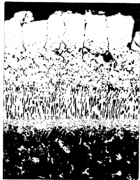
Photo. 5. Cross section of the Al L coating after the hot corrosion test at 750°C. Etching: electrolytically in 10% oxalic acid. (x400x4/5)
