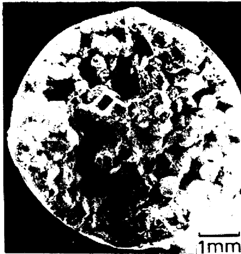
Photo. 6. Fracture surface of SZ after creep rupture testing at 1.9 \text{ kg/mm}^2 in PNP-He at 1000^\circ \text{C} , showing an intergranular fracture.
