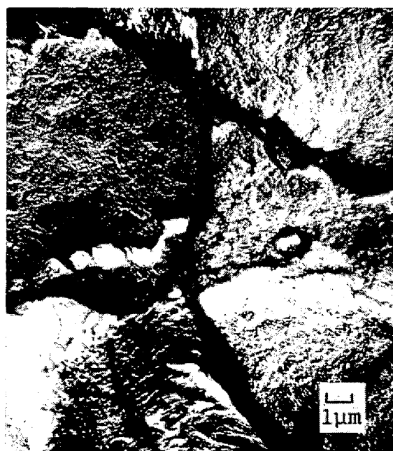
Photo. 1. Fractograph of liquid metal embrittlement cracking of SM50A steel.
