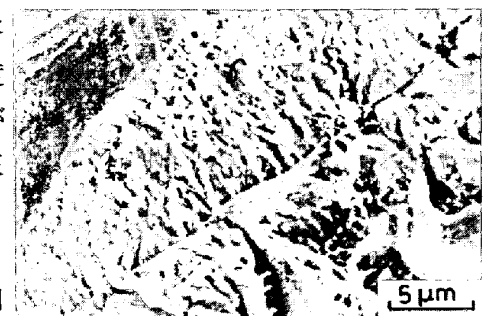
Fig.2 Transgranular cracking in austenite at 50°C
