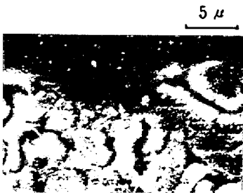
Photo1. Scanning electron micrograph of Coarse carbides on rimmed steel Sheet surface (coiling temp. 650°C)
