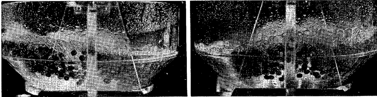
Photo. 1. Typical example of wave motion, which is defined as A type (Gas flow rate; 175NI/ min, Bath depth; 6.8cm, Tuiyere configuration; 「□」 with 18 tuiyeres).
