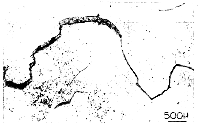
Photo. 1. Photomicrograph of the transverse facial cracks in a continuously cast Al-Si killed steel showing austenite grain boundary fracture.
