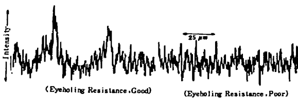
Fig. 3. Cr distribution on the surface of tinplate by EPMA
