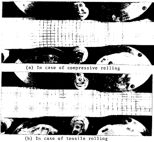
Photo. 1. Deformation of side face of workpiece induced by horizontal 2-stands rolling.
