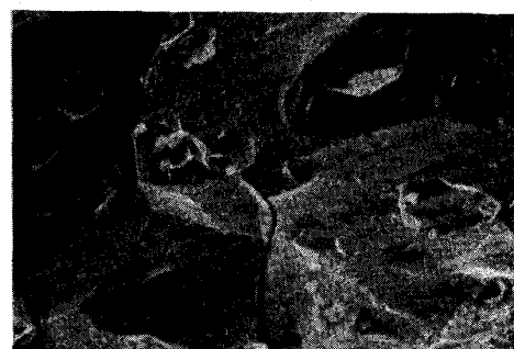
b. IG cracking observed on sensitized 304 under rectangular wave at 2 \times 10^{-4} \text{ Hz} .
