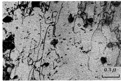
Photo. 6. Transmission electron micrograph of fine precipitation in cold rolled and annealed sheet.
