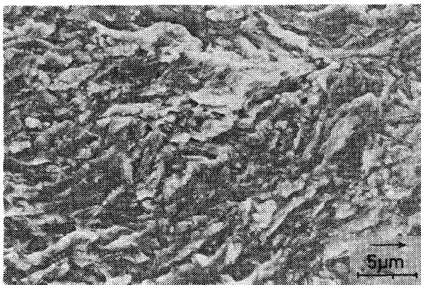
Photo. 4. Example of the fracture surface adhered with corrosion products of HP9-4-20 steel.
