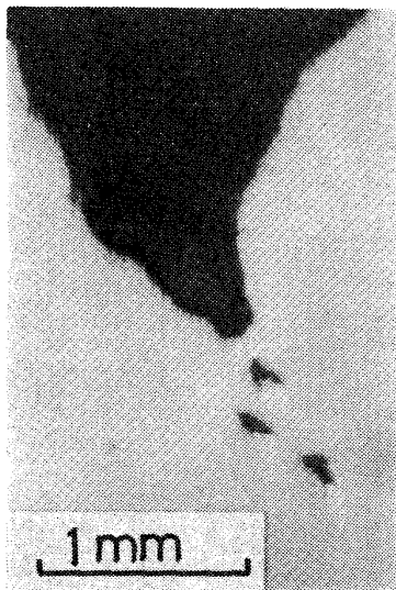
Photo. 4. A longitudinal section showing the formation of microblowholes near the critical small blowhole.
