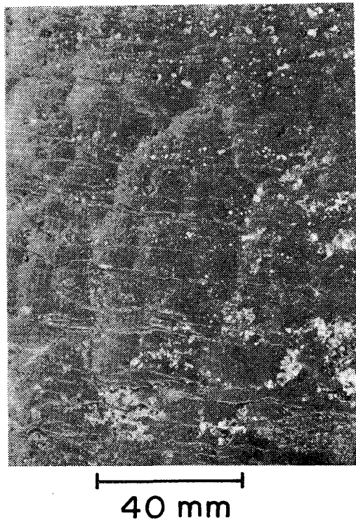
Photo. 2. Surface of shell against water-cooled copper plate.
