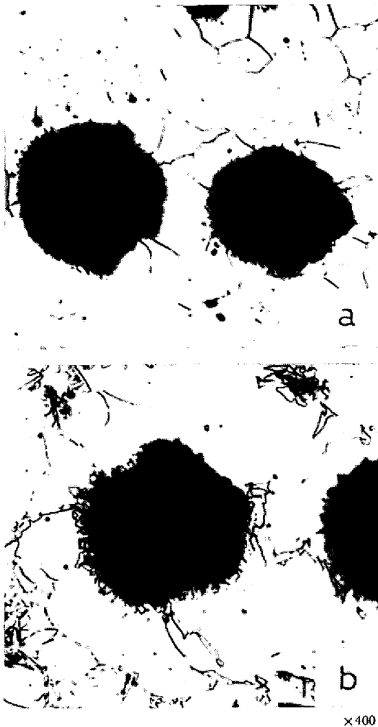
Photo. 2. Change of microstructures during austenitizing (ferritic). (a) as annealed, (b) transformed at 850°C for 10 s.
