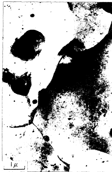
Photo. 1. Transmission electron micrograph showing typical "recrystallized ferrite structure" in Fe-10 Ni-0.2 Nb alloy, cold rolled 80% and annealed at 500°C for 100h. Small austenite grains are seen within or among large recrystallized ferrite grains.
