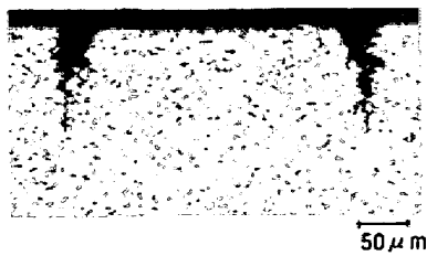
Photo. 4. Stress corrosion cracking observed on bent specimen after constant strain rate test. (2.5h)
