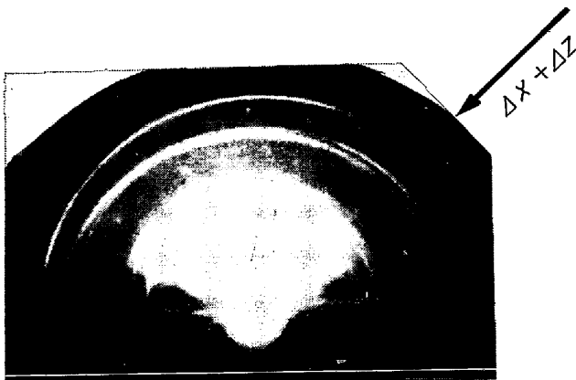
Photo. 6. Double exposure in which Photo. 1 is superimposed on the reference pattern of gold. Ring eccentricity is larger than in Photo. 5, and it is directed other than in Photo. 5. This implies that Photo. 1 is subjected not only to the magnetic field \vec{B} , but also to the electrostatic field \vec{E} at the surface charged with electrons.
