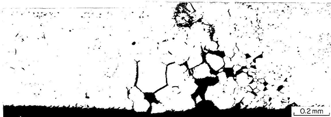
Photo. 4. Intergranular corrosion of B-1 steel (0.026C-0.015N-16.3Cr) in tap water after 14 days immersion.
