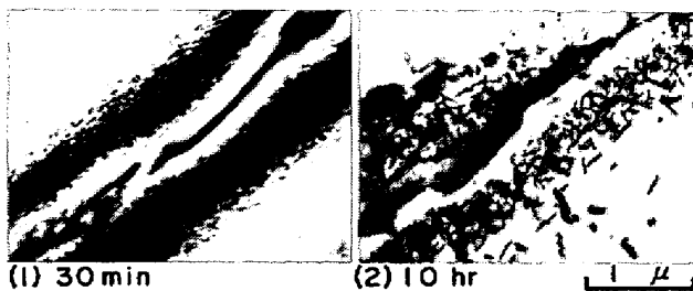
Photo. 6. Electron micrographs of commercial steel A annealed at 600°C after air-cooling from 1 200°C.
